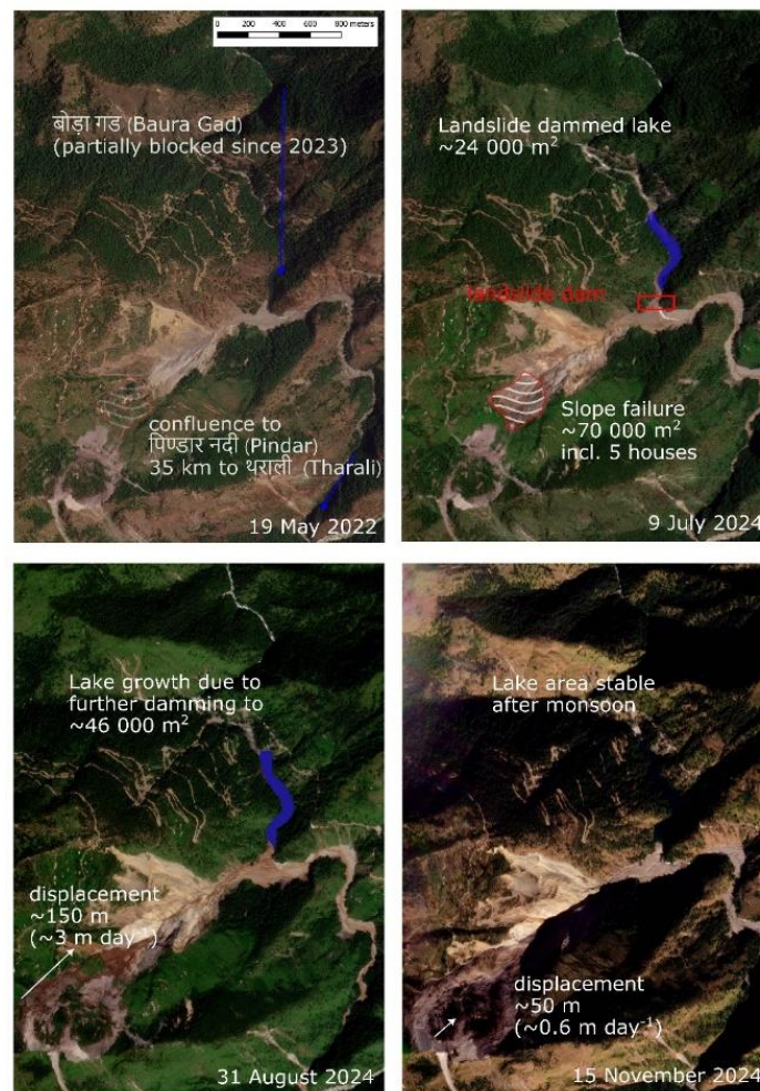
Figure 1: Development of the slope failure since 2022, with the formation of a lake after landslides in 2022, with another significant mass movement during monsoon 2024.
