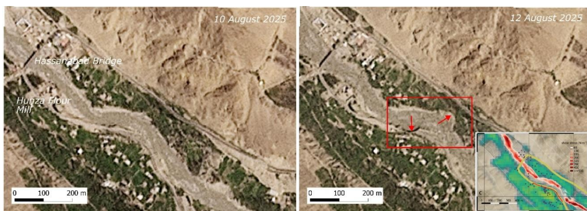
Figure 4: Erosion visible between 10th and 12th August 2025, caused by a flood event from the tunnel collapse at Shisper Glacier. The inset in the second panel, shows GLOF simulation results (shear stress) from 2021 (Muhammad et al., 2021), indicating high shear stress and rapid jumps in stress at the location where erosion is most visible.
