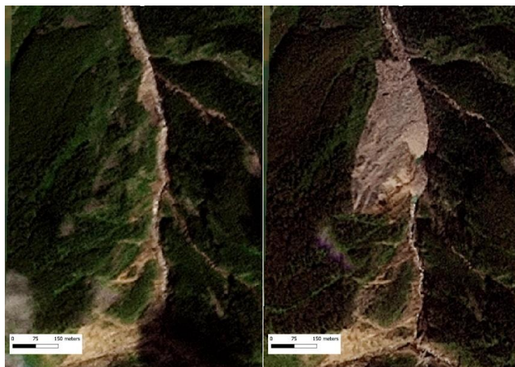
Figure 4: The landslide that formed 1 month after the initial debris flow event in the Thal Gad above Harsil, seen on the 22 nd of August (left) and the 11 th of September (right) on Planet imagery.
